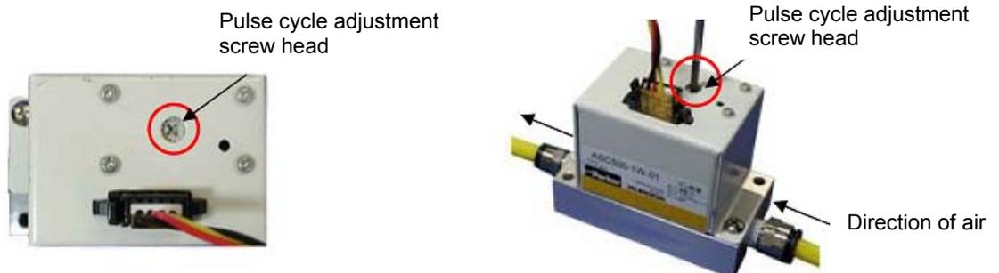
(Reference) Indication for cycle adjustment screw head position and cycle
